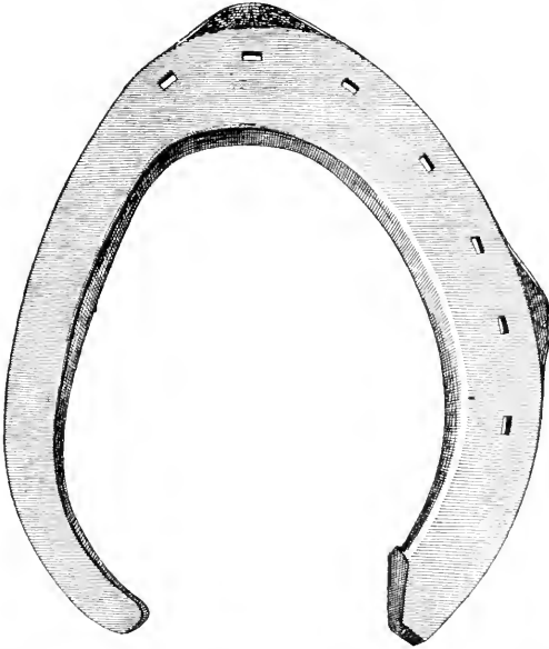
FIG. 13.—Hoof surface of a right hind shoe to prevent interfering. The inner branch has no nail holes and is fitted and beveled under the hoof. Note the number and position of the nail holes, the clip on the outer side-wall, and the narrowness and bend of the inner branch.
